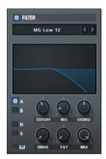
the filter type. Alternatively you can use the < > arrows to the right of the name for advancing through the filter types with a single mouseclick. See the appendix at the very end of this manual for a list of the filter types.
