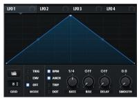
The LFO Module has its own set of controls (pictured) below the (blue) shape. The settings are independent for each LFO. Only the grid size is 'global' to all LFO's.
