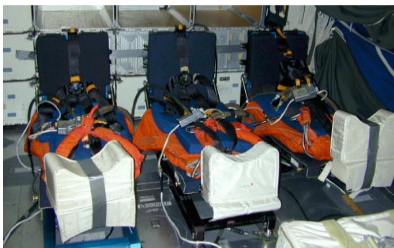
Figure 3-8. MS (PS) seats installed on RSK
