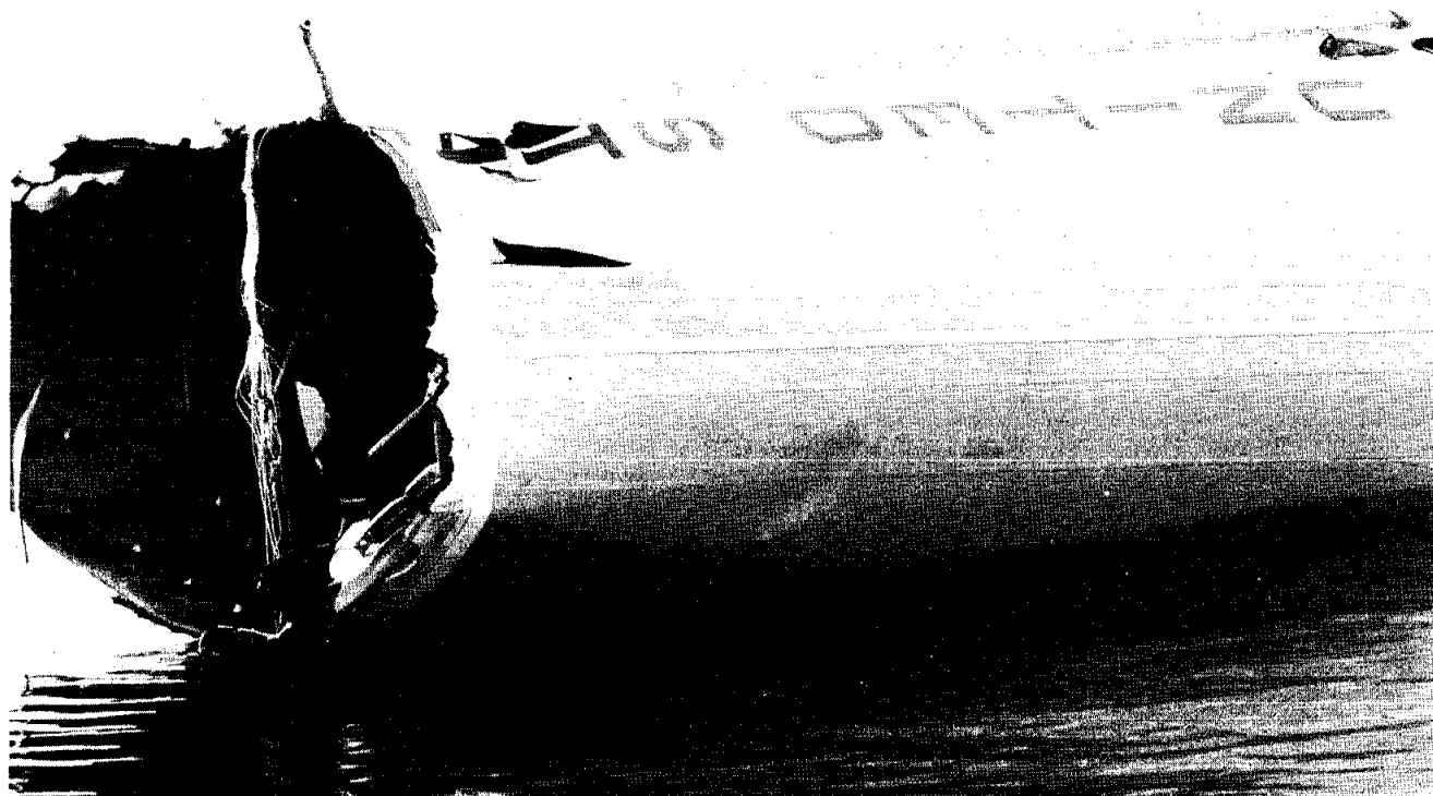
Figure 5.2-2. - Recovered GLV-5 stage I oxidizer tank.
