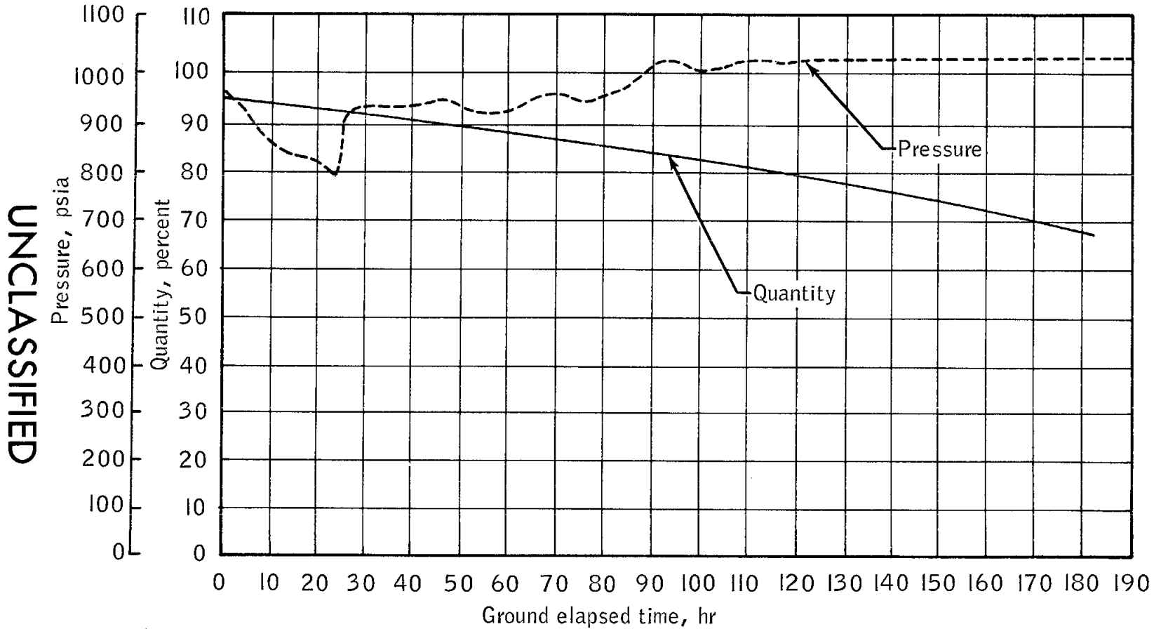
Figure 6.1-3. - Real-time data concerning the ECS primary oxygen supply.
