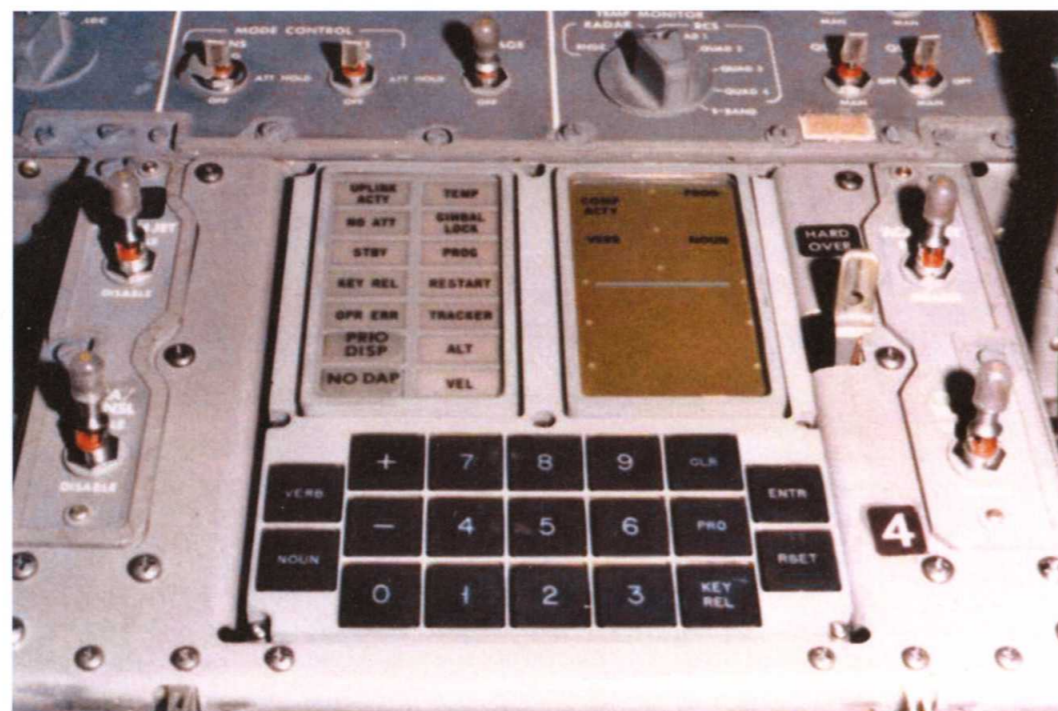
RIGHT The DSKY computer interface inside the Lunar Module. (NASA/Apollo Flight Journal)
