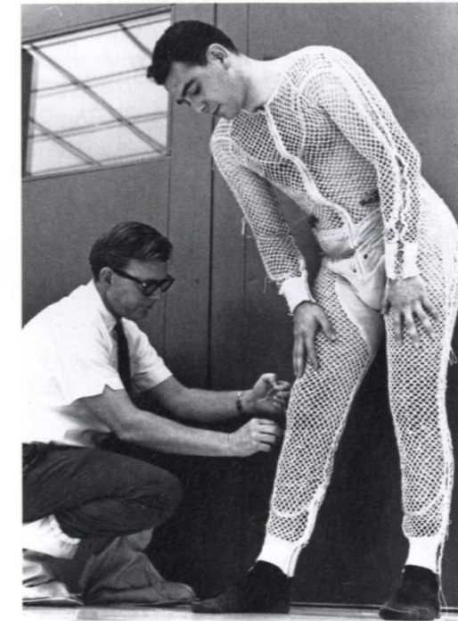
FAR RIGHT AND RIGHT Early evaluation testing of the water-cooled garment concept at Hamilton Standard. (Hamilton Standard)
