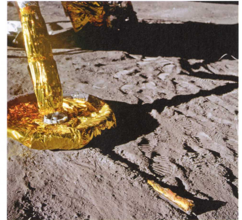
ABOVE The LM 'Eagle' starboard footpad and contact probe on the Sea of Tranquility at mankind's first lunar landing site. (NASA)
