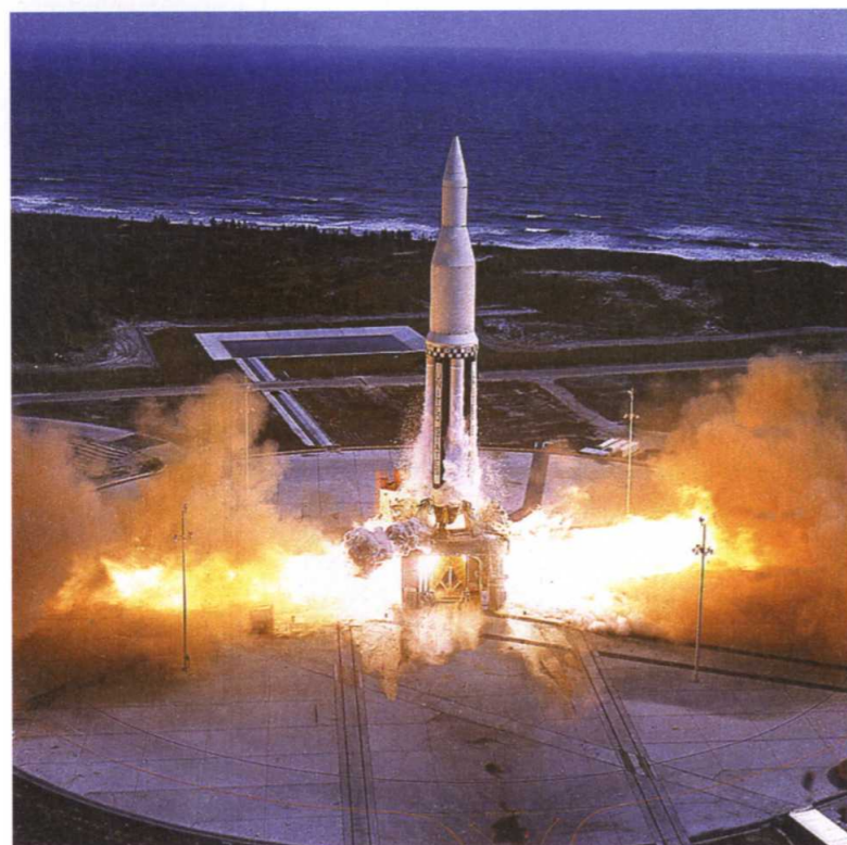
BELOW The Marshall Space Flight Center's first Saturn I vehicle, SA-1, lifts off from Cape Canaveral, Florida, on October 27th, 1961. Weighing 460 tons at launch, this Block 1 first stage was powered by eight H-1 engines. The upper second stage (the S-IV) was a dummy. (NASA/Alan Lawrie)
