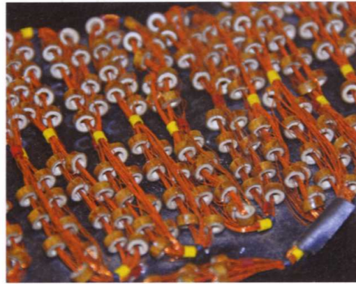
RIGHT Core rope memory used to store software and data on Apollo. (Chris Riley)
