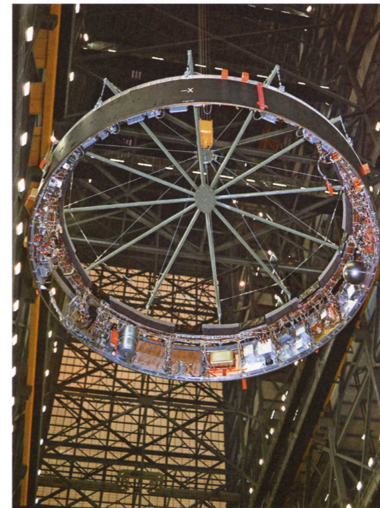
ABOVE This photograph was taken during the final assembly operation of the Saturn V launch vehicle for the Apollo 4 (SA-501) mission. The Instrumentation Unit (IU) is being hoisted to be mated to the S-IC/S-II assembly in the Vehicle Assembly Building high bay at the Kennedy Space Center. (NASA)
