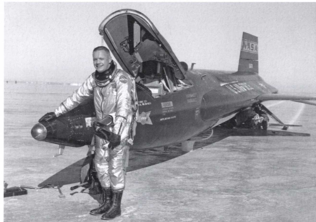
RIGHT Dryden pilot Neil Armstrong is seen here next to the first X-15 after a research flight. The X-15 was a rocket-powered aircraft, 50ft long with a wingspan of 22ft. (NASA)
