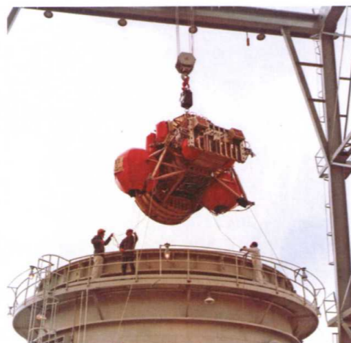
RIGHT Lowering the LM ascent stage onto a testing rig at White Sands for ascent engine test firings. (White Sands Test Facility)
