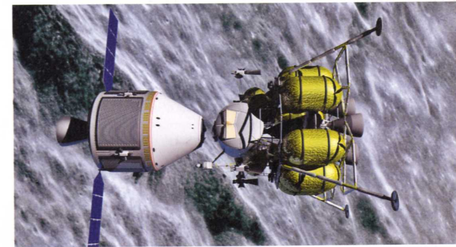
ABOVE Artist's rendering of NASA's new constellation programme, showing a lunar lander undocking from a crew exploration vehicle (CEV) while in Moon orbit. (NASA)
