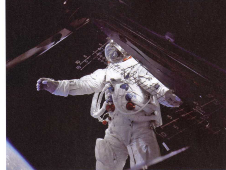
ABOVE Rusty Schweikart stands outside on the LM porch testing the first Apollo pressure suit to be worn in space. He is the first American astronaut to stand remote from his spacecraft in life-support terms. (NASA)
