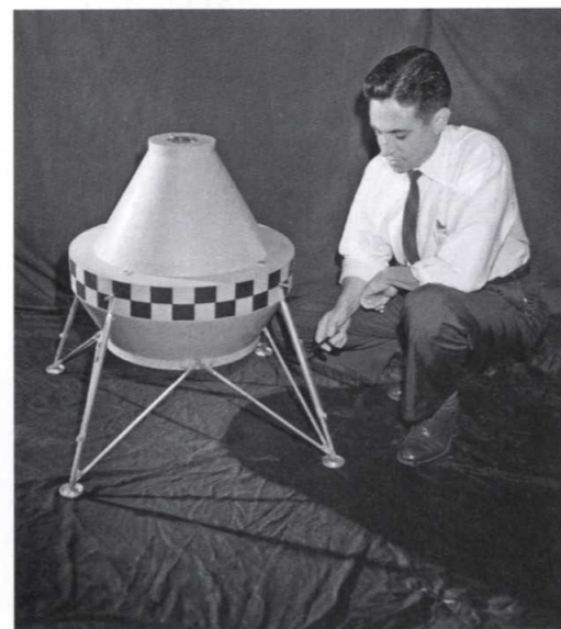
BELOW A scale model of an early prototype Lunar Lander is tested for stability during a simulated landing on soft material. (NASA)
