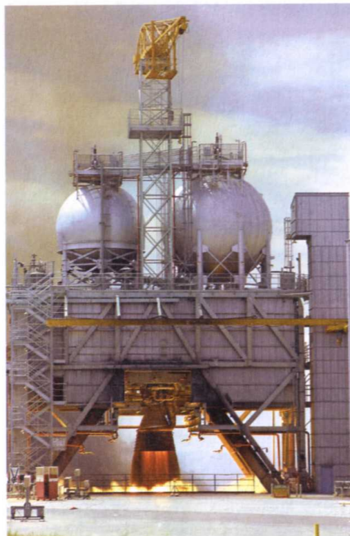
RIGHT Test firing of an F-1 engine at Edwards Air Force Base. (NASA)
