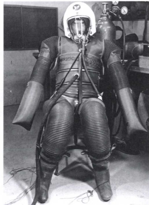
RIGHT An early ILC suit from circa 1955 – demonstrating the rubber convolutes around the elbows, shoulders and legs. A design for a pressure suit glove was still a long way off. (ILC)
