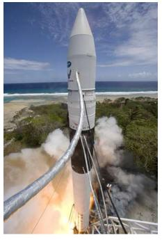
A single SpaceX Merlin 1C regenerative engine powers the Falcon 1 first stage, and is flying in this configuration for the first time on Flight 3. After first stage engine start, the Falcon is held down and not released for flight until all propulsion and vehicle systems are confirmed to be operating nominally.
