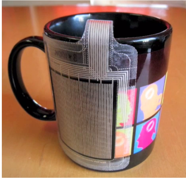
Figure 3.24: IFSR Sensor wrapped around a mug.
