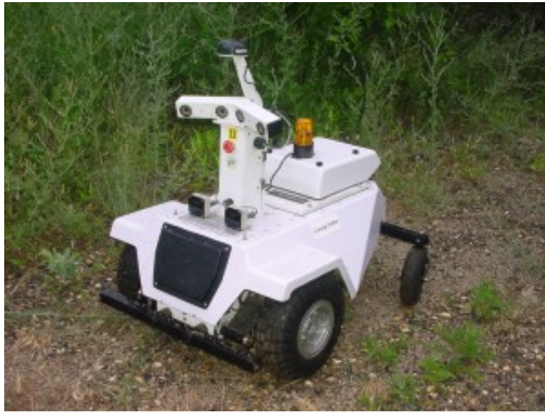
Figure 1.4: One of the autonomous LAGR robots. The SGM algorithm was used to generate ground-truth disparity data to train LAGR’s neural networks for obstacle avoidance.
