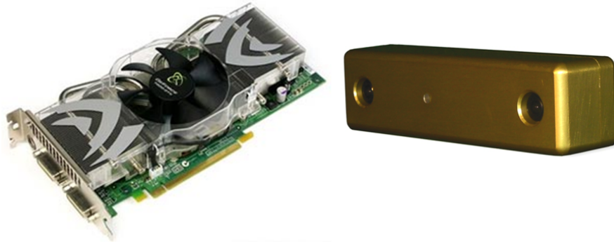
Figure 1.2: We used an nVidia 7900GTX video card to run the SGM algorithm and a Point Grey Research Bumblebee camera to acquire stereo images.
