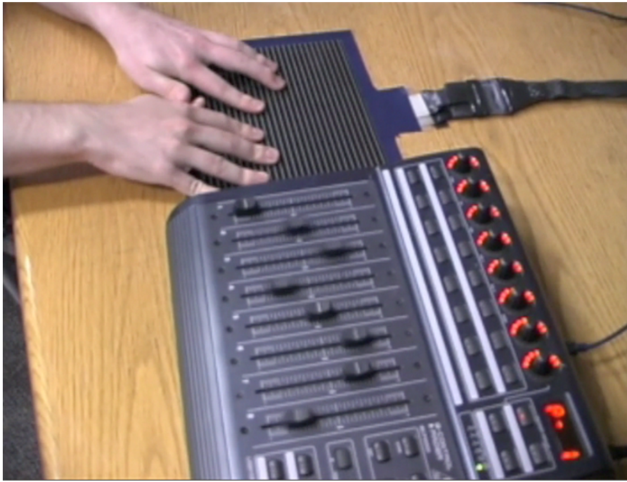
Figure 3.38: Simultaneous isometric control of 8 MIDI faders.
