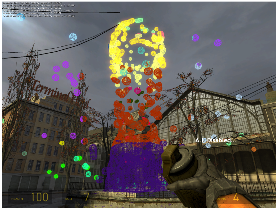
Figure 2.7: This simulated fountain is too big to render in a single marching cubes volume, so it is seamlessly split into multiple blocks, which are shown here in different colors.
