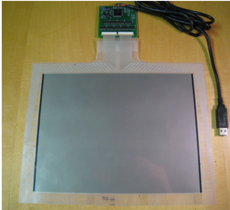
Figure 3.5: 8.5" x 11" UnMousePad with drone wires
