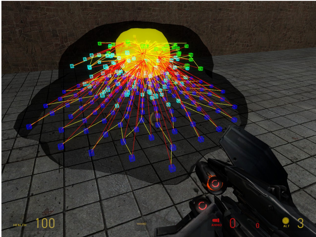
Figure 2.15: Procedural animation of blob monster. Squares represent particles, and the color of the square represents the particles function (yellow particles belong to the brain, light blue particles are structural, dark blue particles are feet, and green particles are arms). Yellow lines show the tree structure of the blob, and red lines represent “tendons” which apply forces to hold the blob together.
