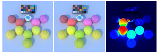
Figure 11: The effect of including UV radiation in outdoor renderings that feature fluorescent surfaces. The inner objects have diffuse fluorescent BRDFs with measured re-radiation data of real materials. On the outer objects, only the non-fluorescent main diagonal of the same measurements is used. A significant number of fluorescent surfaces re-radiate energy from both the short-wavelength visible and the near UV ranges to longer wavelengths, and omitting UV irradiance alters their appearance. Illumination is with the proposed skylight model, turbidity 3. Left: 8 spectral samples, without UV Middle: 16 samples, with UV - notice how the leftmost two fluorescent surfaces gain in chroma Right: \Delta E difference image
