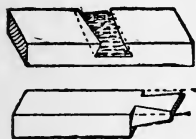
Fig. 48.—Bevelled Dovetail Half- lapped Joint.
