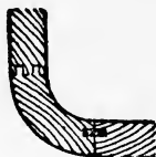
Fig. 110. Single Loose Tongue and Double- tongue Joint.
