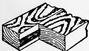
Fig. 101.—Joint with Single Dovetail Tongue and Groove.
