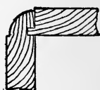
Fig. 116. Corner Joint with Corner Mould.
