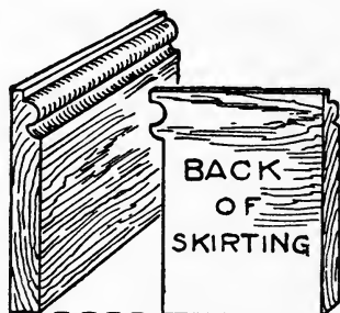
Fig. 369.—Scribing Joint on Skirting Board.
