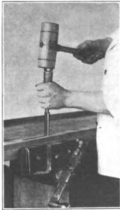
FIG. 261. LAST STEP IN MORTISING.
