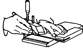
FIG. 339. CUTTING ACROSS THE GRAIN.
