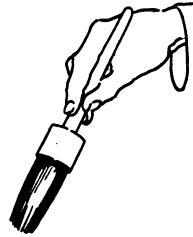
FIG. 376. CORRECT METHOD OF HOLDING BRUSH.
