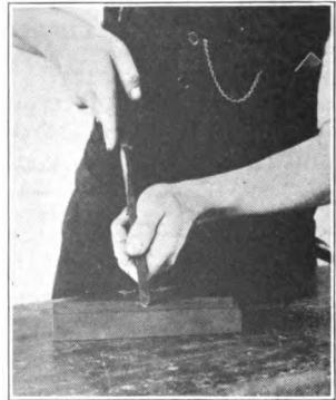
FIG. 53. PUTTING BURR ON SCRAPING CHISEL.
