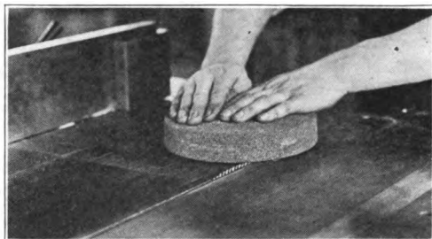
FIG. 177. JOINTING CIRCULAR SAW TEETH.
