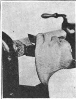
FIG. 296. USING LARGE SKEW—SECOND POSITION.
