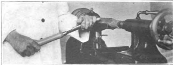
FIG. 289. POSITION OF HANDS ON GOUGE—FIRST POSITION.
