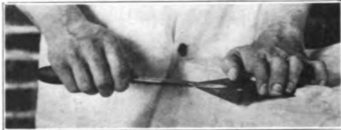
FIG. 122. DRAWING OUT BURR ON SCRAPER.
