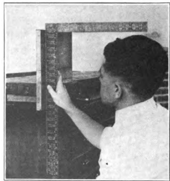
FIG. 250. TESTING FACES OF GLUE JOINT.
