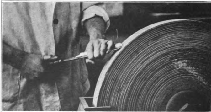
FIG. 123. GRINDING A TURNER'S GOUGE.
