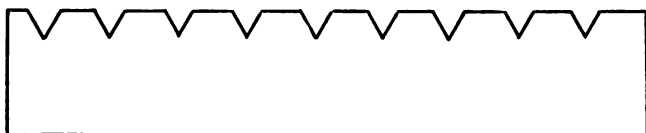
FIG. 231. LINER FOR BABBITTING BEARINGS.
