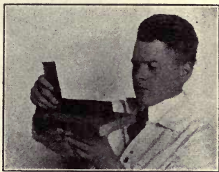
Fig. 59. Fourth Test for Surface Trueness
