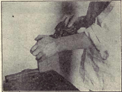
Fig. 54. End Planing; Second Position
