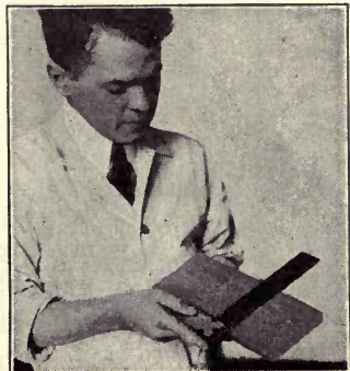
Fig. 19. Test for Uniformity of Width
