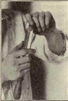
Fig. 91. Thumb-nail Test for Sharpness
