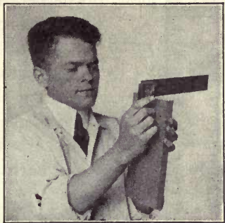
Fig. 17. Testing End for Squareness
