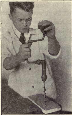
Fig. 69. Vertical Boring; First Position
