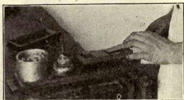
Fig. 87. Starting Position in Whetting
