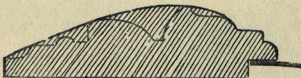
FIG. 43.—SECTION OF SHAPED MOULDING
