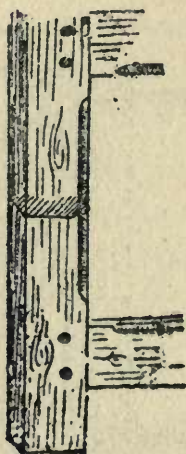
FIG. 67.—MOULDED STILE AND RAIL
