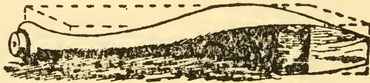
FIG. 95.—CABRIOLE LEG FINISHED.
