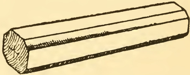
FIG. 6.—PIECE OF WOOD WITH CORNERS ROUGHLY PLANED AWAY READY FOR MOUNTING BETWEEN THE LATHE CENTRES.
