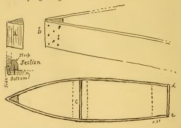
The simplest kind of a craft is the best to start with. Get two boards, smooth and with as few knots as possible, 15 in. wide, and 15 ft. long; about 50 sq. ft. of tongue and groove flooring; a piece of 2 x 6 in. scantling, 15 in. long; and plenty of 3-in. nails.
