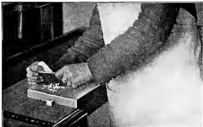
FIG. 82.—METHOD OF GRASPING THE SCRAPER WHEN WORKING UPON A BROAD SURFACE.
