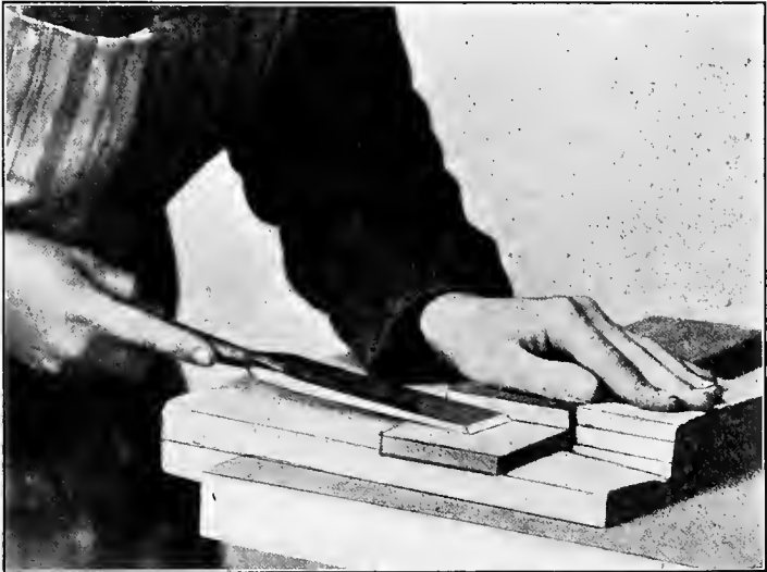
FIG. 117. — USE OF THE BENCH HOOK WITH THE PARING CHISEL.
