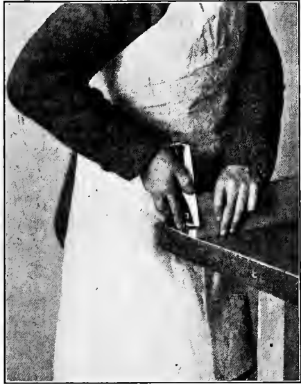
FIG. 58.—USING BLOCK PLANE UPON SMALL PIECES.
