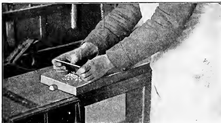
FIG. 83.—METHOD OF GRASPING THE SCRAPER WHEN WORKING WITHIN A SMALL AREA.
