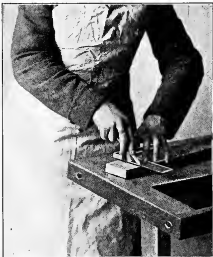
FIG. 31.—POSITION OF TRY-SQUARE WHEN MAKING LINE.
