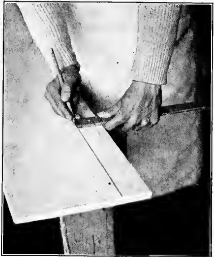
FIG. 114.—LINING OFF FOR RIPSAWING.
