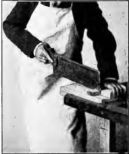
FIG. 115.—USE OF THE BENCH HOOK AND THE BACKSAW.
