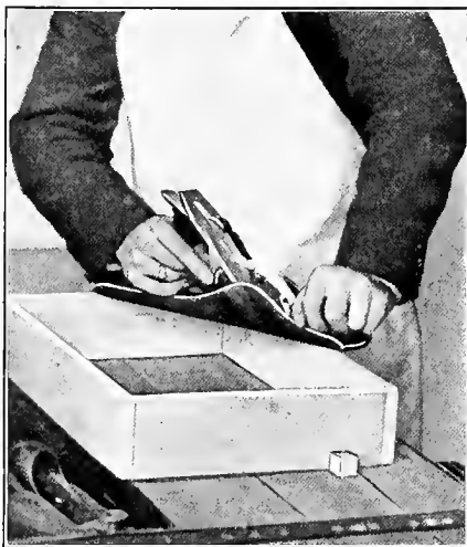
FIG. 187. — PLANING THE EDGE OF A BOX TO FIT THE BOTTOM.
