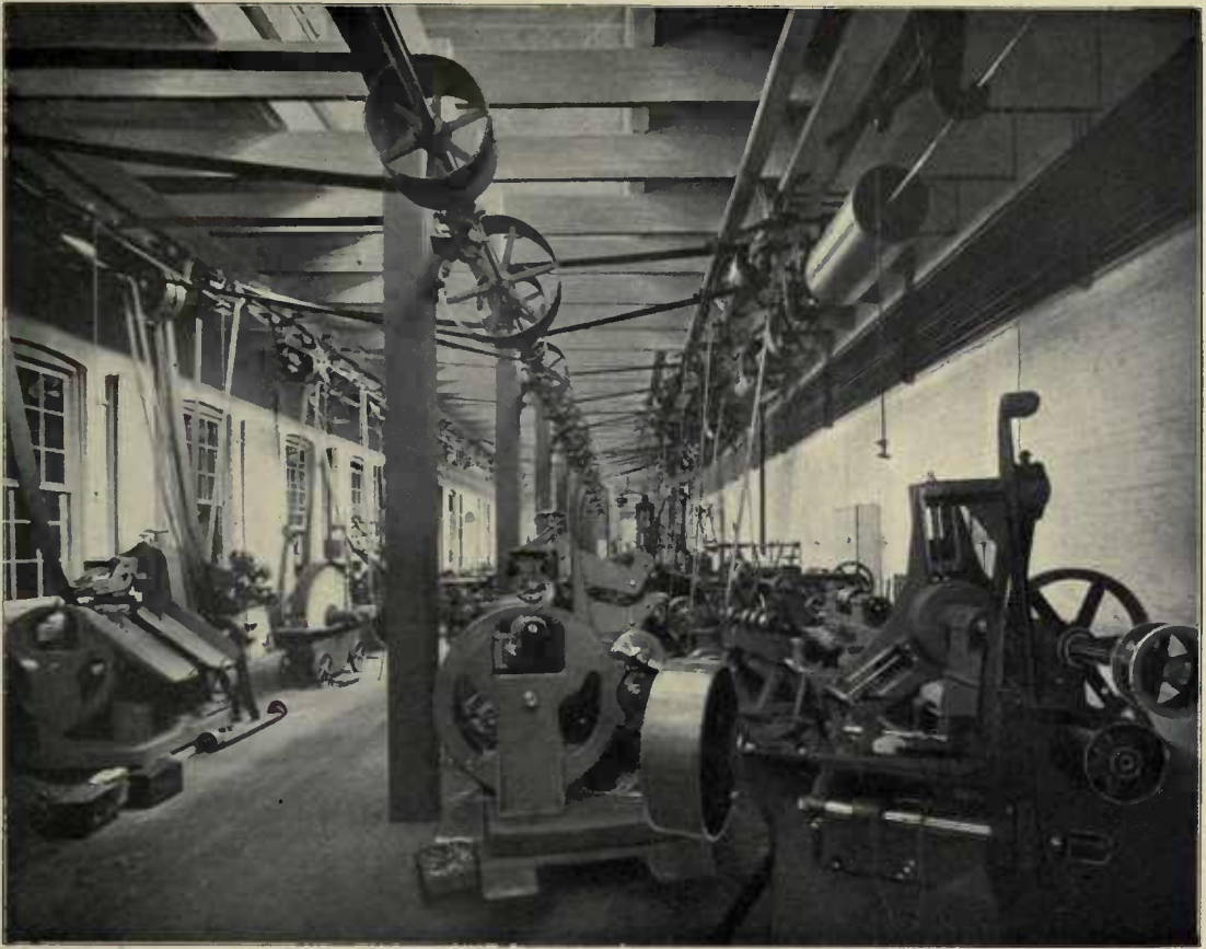
TESTING ROOM—WHERE EACH MACHINE IS PUT TO ACTUAL TEST BEFORE SHIPMENT IS MADE.
