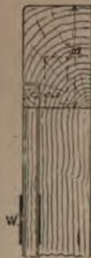
Fig. 738.—Section of Bed-frame showing Webbing.
