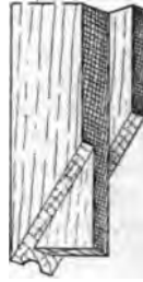
Fig. 1396.—Mitered and Rebated Frame of Flower Stand Top.
