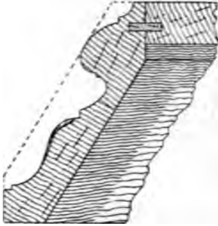
Fig. 175.—Enlarged Section through Part of Dinner Waggon Bottom.
