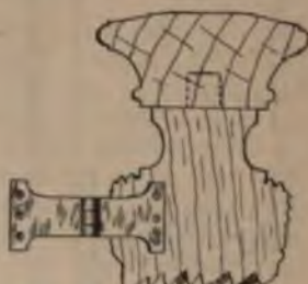
Fig. 1791.—Section of Rail showing Top Hinge.
