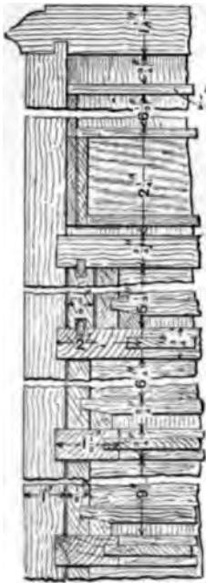
Fig. 862.—Vertical Section of Bureau Side, etc.
