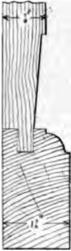
Fig. 942.—Section of End Panel Framing of Writing Table and Cabinet.
