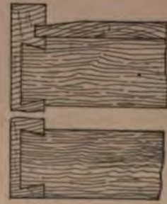
Fig. 616.—Joint of Top Rails of Dressing-chest.
