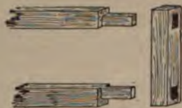
Fig. 1490.—Joint of Curio Table's Side Framing.
