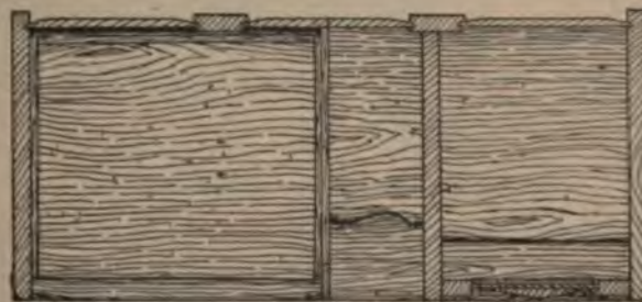
Fig. 631.—Half Horizontal Section of Modern Washstand.
