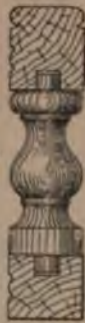
Fig. 826.—Cross Section of Desk Rails, and Spindle on Line E E (Fig. 819).
