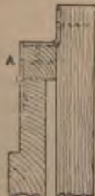
Figs. 1154 and 1155.—Part Sections through Back, Top, and Hanging Fillet of Collapsible Cupboard.
