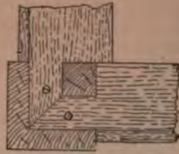
Fig. 975.—Joint of Top Rails and Leg of Writing Table.
