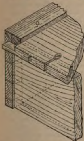
Fig. 934.—Part View of Back of Pedestal Drawer.
