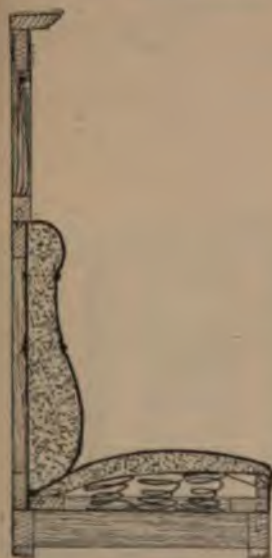
Fig. 1534.—Section through Seat and Back of Cosy Corner Settee.
