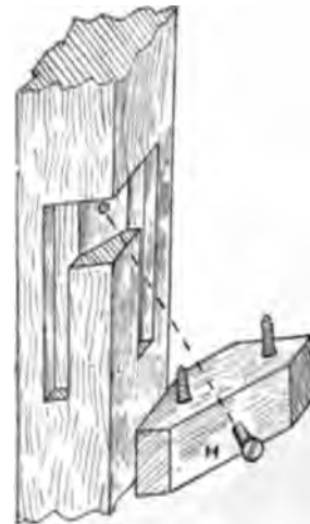
Fig. 1389.—Housing in Palm Stand Leg for Shelf Rails.
