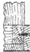
Fig. 802.—Horizontal Section through fixed Plaster of Right-hand Pedestal on Line G G (Fig. 794).
