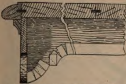
Fig. 205.—Enlarged Section of Overmantel Base on Line G G (Fig. 203).
