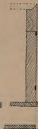
Fig. 1477.—Section of Drawer End of Box.
