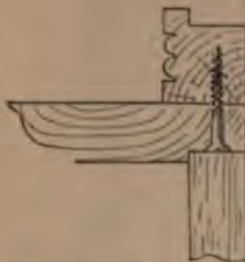
Fig. 1604.—Section of Mirror Frame and Shelf on Line B B (Fig. 1600).
