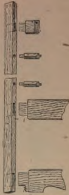
Fig. 1316.—Joints in Screen Framing.
