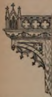
Fig. 1780.—End Elevation of Choir Stalls Canopy.
