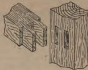
Fig. 477.—Double-tenon between Drawer Framing and Post of Music Stool.
