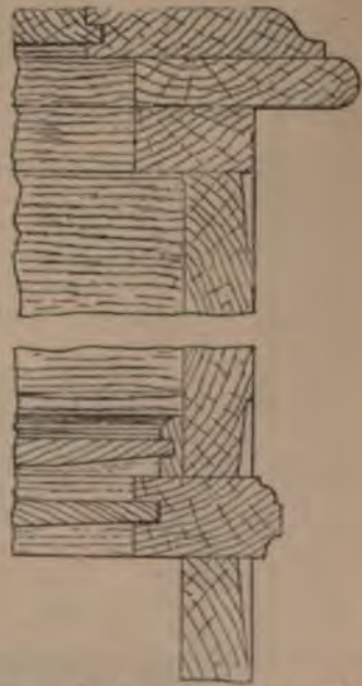
Fig. 825.—Cross Section through Drawer Fronts, etc. (see D, Fig. 820).
