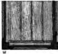
HALF HORIZONTAL SECTION AT Y, SHOWING COMPARTMENTS FOR MUSIC.
