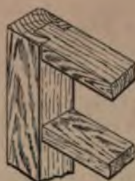
Fig. 1006.—Front Rails of Desk Jointed to Leg.
