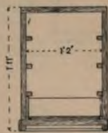
Fig. 922.—Vertical Section through Drawer Carcase of Draughtsman's Table.
