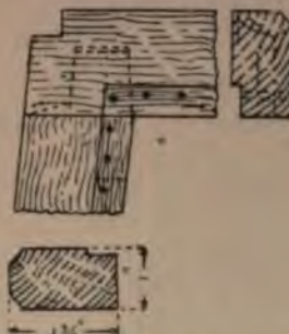
Fig. 599.—Joint in Chair Seat Frame (C, Fig. 598).
