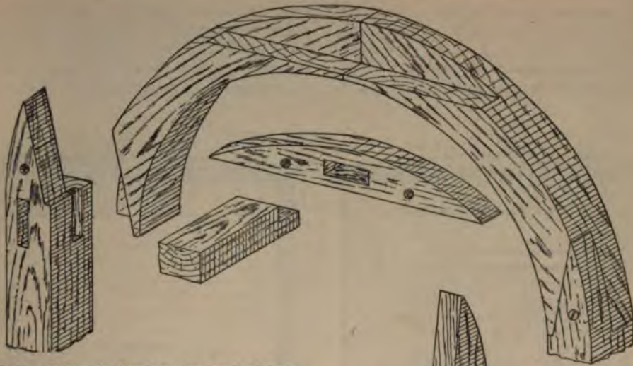
Fig. 1060.—Joints in Semicircular End of Safe.
