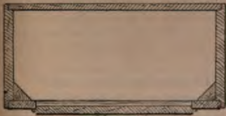
Fig. 1957.—Horizontal Section of Grandfather Clock Case at A (Fig. 1955).
