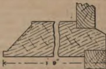
Fig. 135.—Section through Top of Sideboard.
