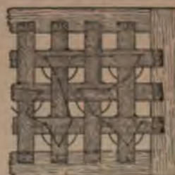
Fig. 1530.—Part Underneath View of Seat Frame of Cosy Corner Settee.
