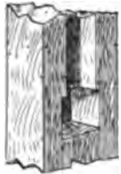
Fig. 1340.—Grooving Screen Rails and Posts for Panels.
