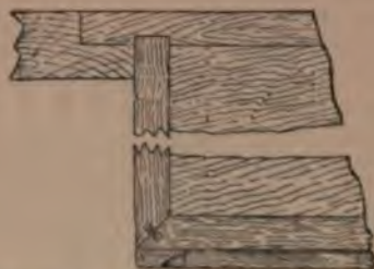
Fig. 1595.—Part Horizontal Section of Glove-box of Mirror.
