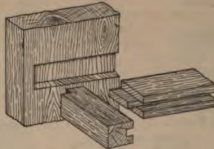
Fig. 617.—Fixing Framing of Dressing-chest Rails and Bearers.
