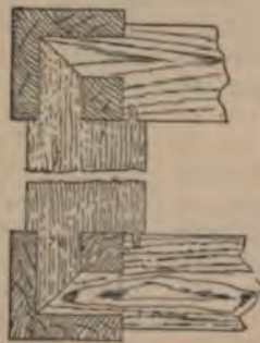
Fig. 977.—Section of Corner Legs and Rails of Writing Table.
