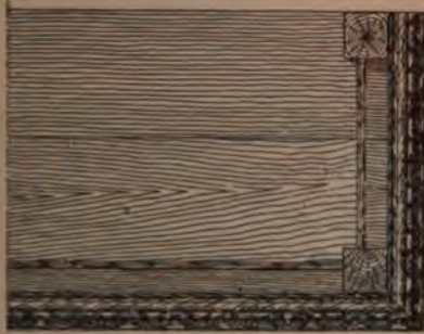
Fig. 171.—Half Horizontal Section of Dinner Waggon through Shelf Level.
