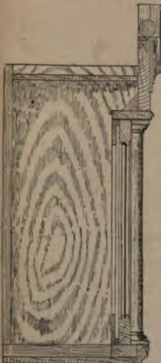
Fig. 1963.—Vertical Section through Centre of Top of Clock Case.
