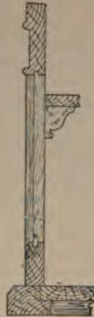
Fig. 1771.—Section through Front Framing of Choir Stalls.
