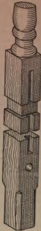
Fig. 681.—Corner Washstand Post cut to receive Rail (see B and C, Fig. 678).
