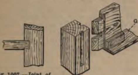
Fig. 1008.—Joint of Side Rail to Leg of Desk.
