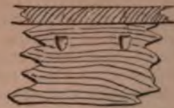
Fig. 996.—Securing Top of Writing Table.
