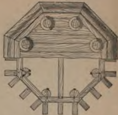
Fig. 1852.—Half Plan of Pulpit Base and Half Horizontal Section at B (Fig. 1850).
