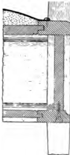
Fig. 470. Part Cross Section of Music Stool Seat, etc., at J (Fig. 464).
