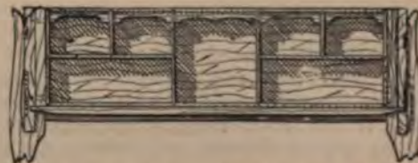
Fig. 998.—Vertical Section of Table (at B, Fig. 990) showing Pigeon-holes.
