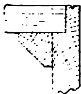
Fig. 697. Fitting Side of Commode to Back.
