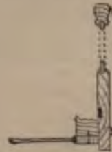
Fig. 1857.—Section of Pulpit Handrail, String, and Soffit.
