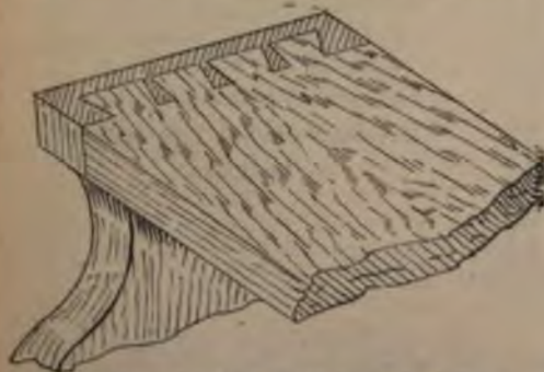
Fig. 1924.—Joint of Shelf to End of Rack.
