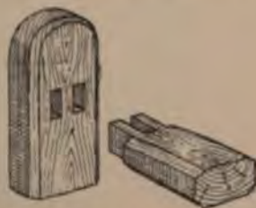
Fig. 1709.—Joint in Linen Press at A (Fig. 1699).
