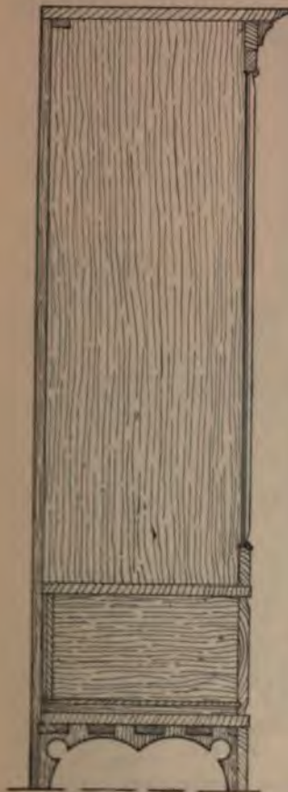
Fig. 604.—Cross Section of Modern Wardrobe.
