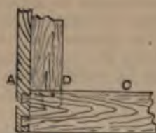
Fig. 455.—Top Drawer Divisions of Combined Cabinet and Table Dovetailed to Gables.
