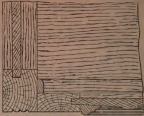
Fig. 824.—Horizontal Section of Part of Desk Cupboard on Line C (Fig. 819).
