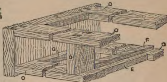
Fig. 1045.—Rails, Divisions, etc., of Dresser.
