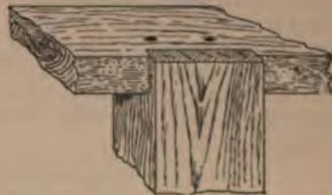
Fig. 976.—Joint of Front Rail and Middle Leg of Writing Table.
