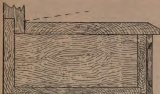
Fig. 1594.—Vertical Cross Section through Glove-box of Mirror.
