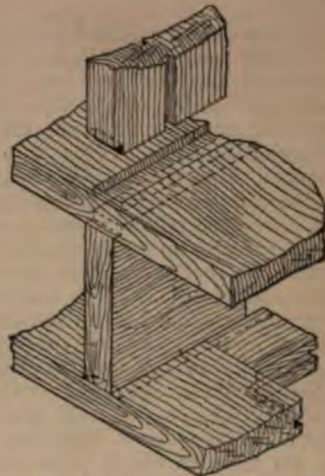
Fig. 130.—Part of Sideboard Drawer Rails and Partitions.
