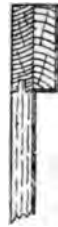
Fig. 805.—Horizontal Section through Pilaster fixed to Door of Left-hand Pedestal on Line F F (Fig. 794).
