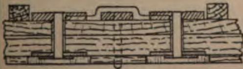
Fig. 1446.—Vertical Section of Jewel Casket Lock in Position.
