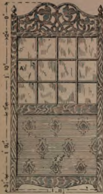
Fig. 1314.—Elevation of Room Screen.
