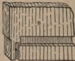
Fig. 931.—Method of Fitting Plinth to Pedestal.
