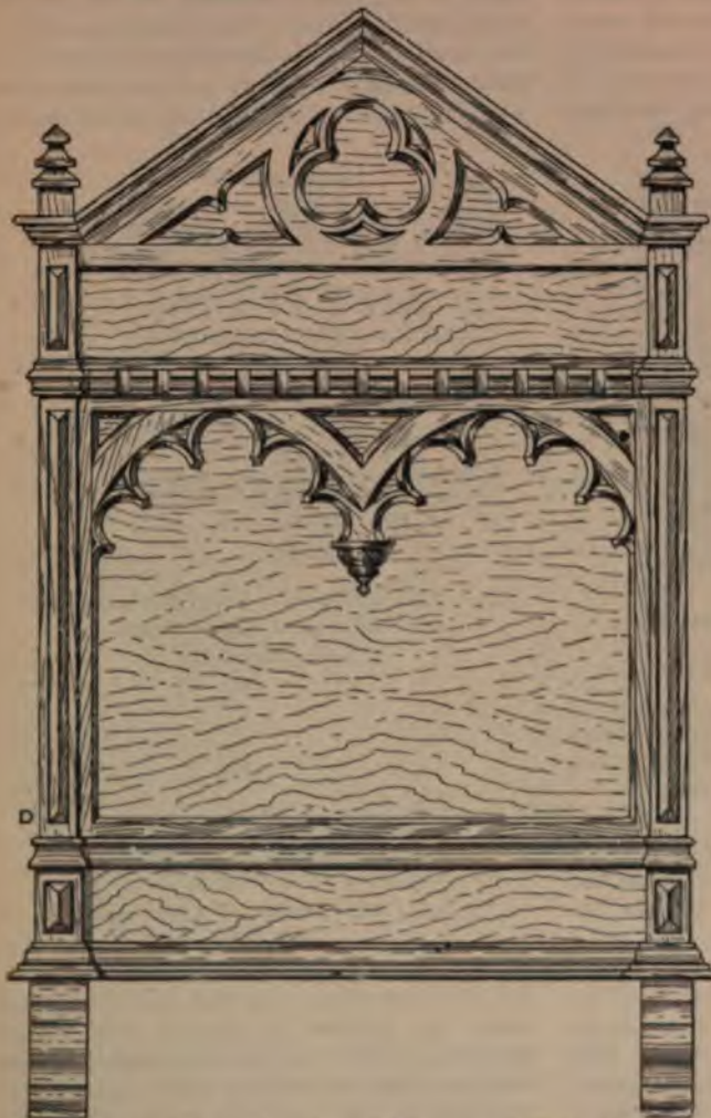
Fig. 1735.—Front Elevation of Three-panel Notice Board.
