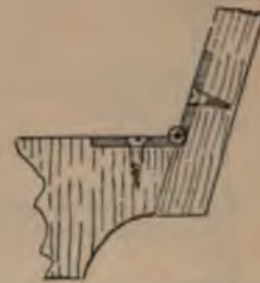
Fig. 1927.—Hinged Joint for Wings of Newspaper Rack.
