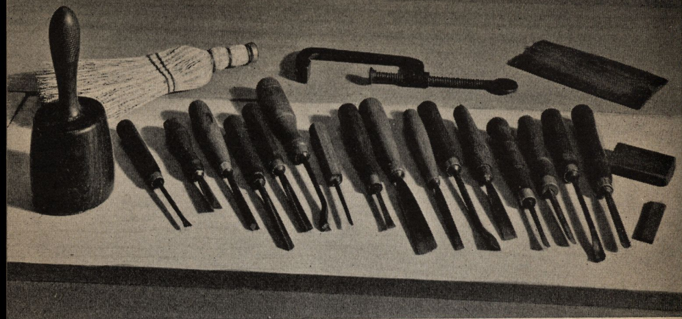
The kit, as recommended on page 9. The skew chisel (No. 1) is on the left and the fluter (No. 16) on the right.
