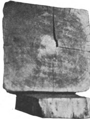
FIG. 32.—The same section of Eucalyptus log as shown in Fig. 31 after being in water for three weeks. The cracks have mostly closed up, but the right-hand top corner broke off when being lifted out of the water.
