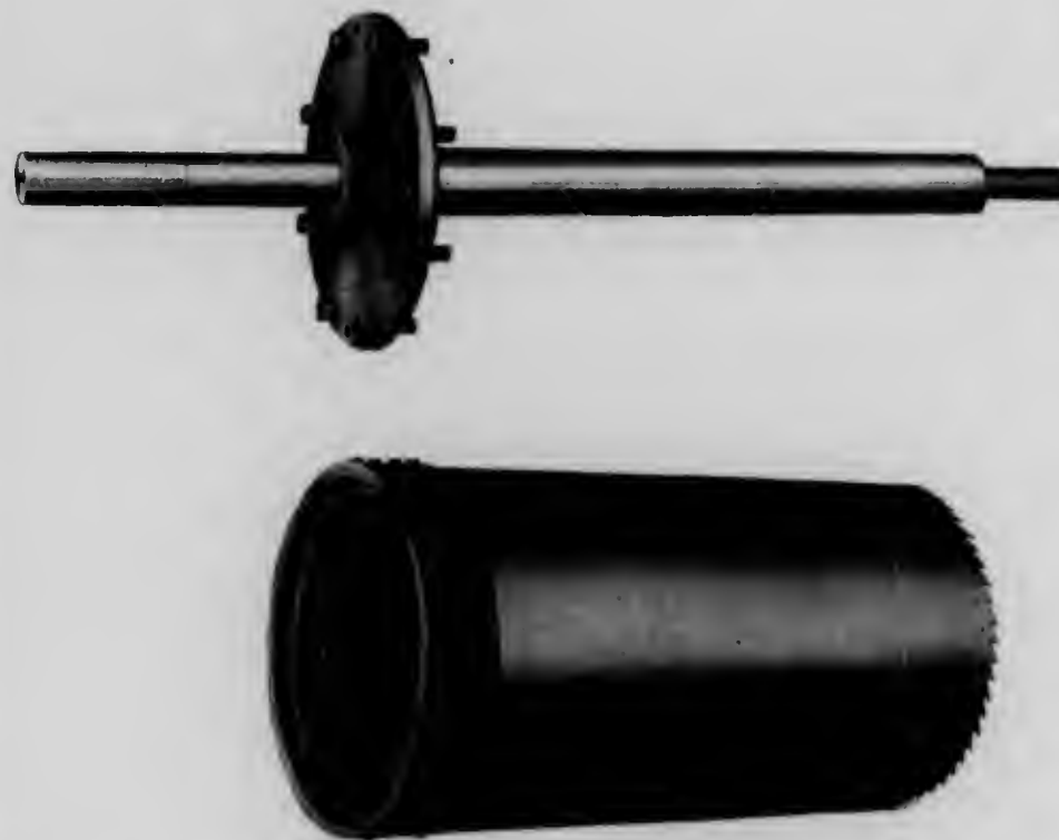
DETACHABLE SAW DRUM FOR WHITNEY STAVE-SAWING MACHINE
