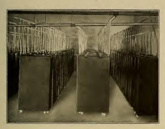
Showing oxygen cell plant making 99% purity oxygen from water by electrolysis.
