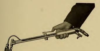
Cutting torch which cuts steel 2" thick x 1 ft. wide in 1 minute; or cuts a battleship slab of steel 4 ft. x 4" in 7 minutes.
