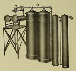
Cut showing chemical oxygen plant, which we do not recommend only in emergency cases as the gas is not as pure. 1 foot of Electrolytic oxygen gas goes as far as 2 feet of Chemical gas in cutting and same pro rata in welding.
