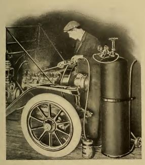
Oxygen Carbon Burner at Work.
