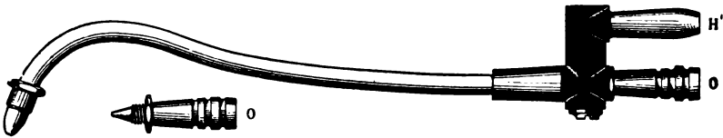
FIG. 29.—Oxy-Coal Gas Blowpipe.
