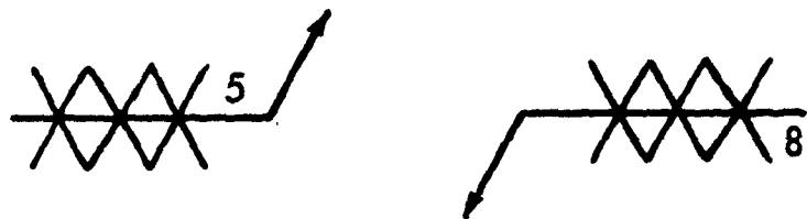
C —LENGTH OF RESISTANCE SEAM WELDS
