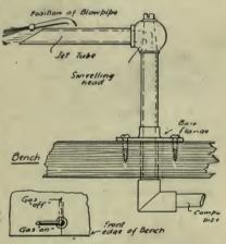
Fig. 29.—Swivelling Gas-burner for Bench Soldering
