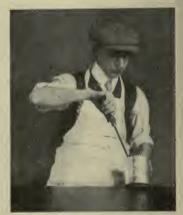
Fig. 21.—Soldering on Can Bottom Internally
