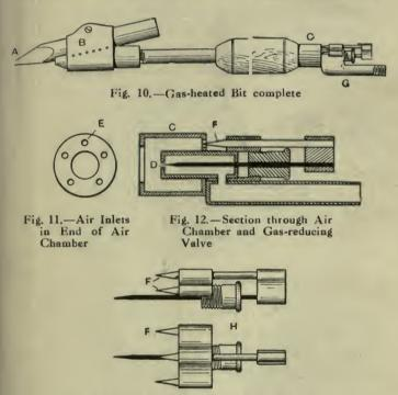
Fig. 13.—Details of Cones or Needles
