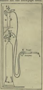
Fig. 72. — Diagram of Oxyacetylene Welding Apparatus
