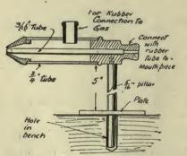
Fig. 31.—Gas Blowpipe for Bench
