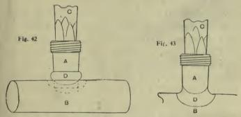
Figs. 42 and 43.—Soldered Branch Joint on Tin or Compo. Pipe
