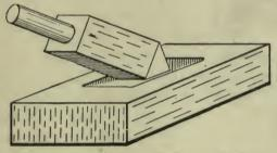
Fig. 16.—Tinning Bit in Sal-ammoniac Block
