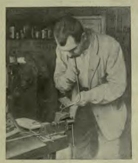
Fig. 37.-Soldering Wires of Vegetable Masher
