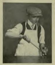
Figs. 18 and 19.—Incorrect and Correct Methods of Holding Bit
