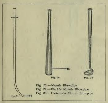
candle, or a methylated-spirit flame. Three shapes of mouth blowpipe are shown in Figs. 23 to 25. In a blowpipe flame there are three cones, X, Y, Z (Fig. 26). X is a non-luminous cone, consisting of a mixture of atmospheric air and unburnt combustible gases (each with a low temperature); Y is a luminous cone, composed of burning gases (carbon and carbonic acid being in excess); and Z is a cone the oxygen in which renders it less luminous and free from com-
