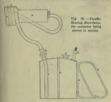
and sweated in beneath. This is passed through a hole drilled in the lid for its reception, and the base of the cock is then sweated in position. Note that the length of this pipe is such that when the lid is in place it clears the container bottom by  $\frac{1}{8}$  in.
