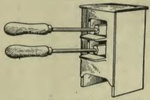
Fig. 15.—Gas-stove for Heating Bits
