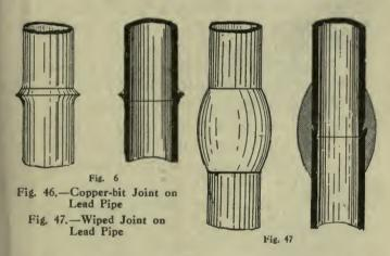
the solder be heated to redness, as the tin rises to the top and quickly turns to dross (see p. 11). If this should happen to solder that is being used for service pipes, it should be rectified by adding more tin.
