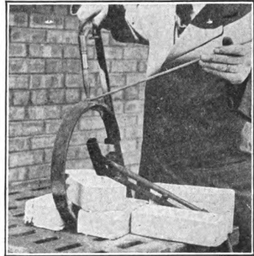
Fig. 38. Gas Burner for Pre-Heating
