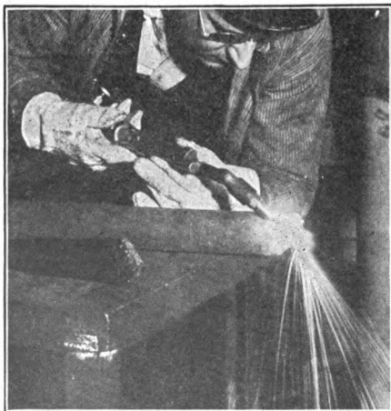
Fig. 80. Beveling Round Shaft for Welding. The other piece is on the table
