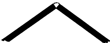
Fig. 54. Broad Corner Weld for Light Sheets
