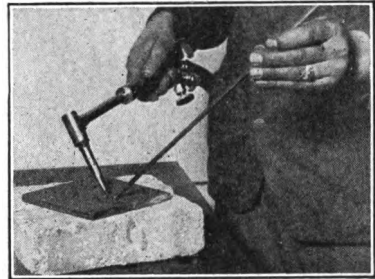
Fig. 25. Correct Method of Holding Welding Rod
