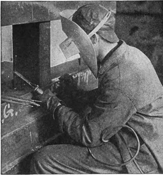
Fig. 12. Operator Using Metallic Electrode Courtesy of C & C Electric and Manufacturing Company, Garwood, New Jersey
