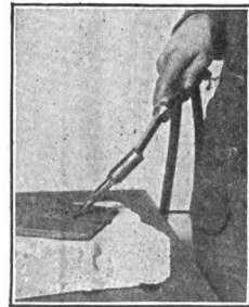
Fig. 22. Blowpipe Should Not Travel Backwards
