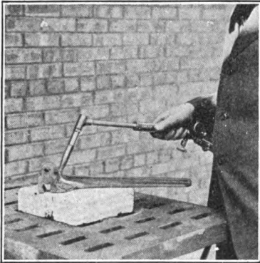
Fig. 37. Pre-Heating with Welding Blowpipe
