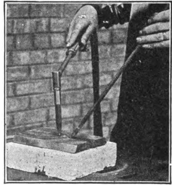
Fig. 76. Welding Rod Should Not Be Held Too Far from Welding Zone.
