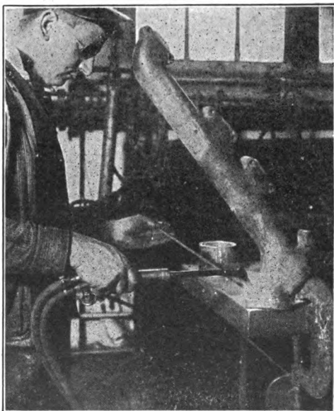
Fig. 100. Welding Broken Flange on Manifold
