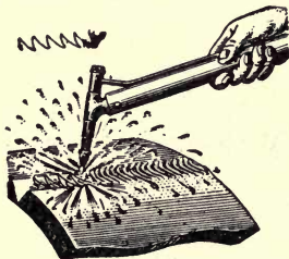
Figure 71.—Oscillatory Movement for the Execution of Welds of Great Thickness
