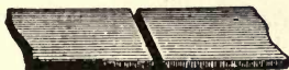
Figure 62.—Beveling for Pieces from \frac{1}{8} inch to \frac{3}{16} inch in Thickness, Angle of Bevel, 45^\circ
