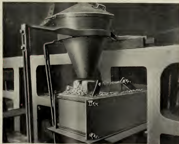
READY FOR POURING. Crucible and sand box surrounding fire brick mold in position.
