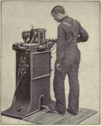
Fig. 3. Hand-operated Machine with Output of 250 Welds on Straight Stock with Welding Area Equivalent to <sup>3</sup>/<sub>4</sub>-inch Round Cross-section
