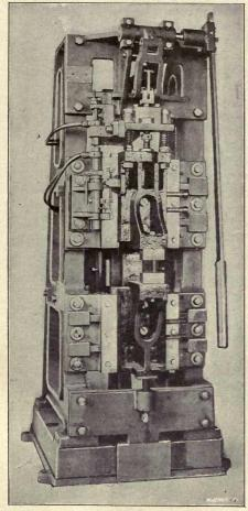
Fig. 3. Type of Electric Welding Machine for Heavy Work
