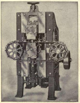
Fig. 4. Automatic Electric Sheave Welder
