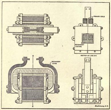
Fig. 1. Typical Transformer for Welding Machines
