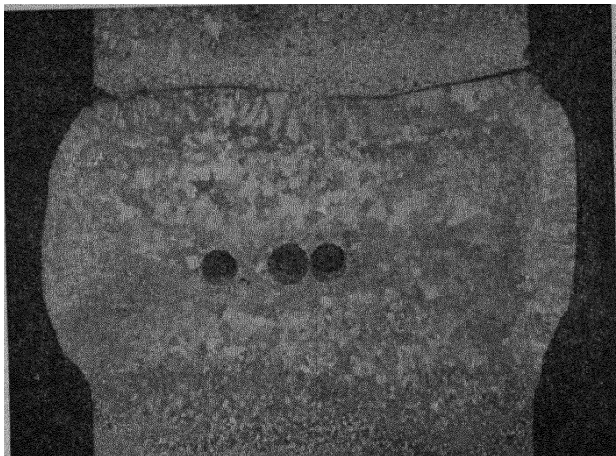
Fig. 206. Gas pockets in electric slag weld made with damp flux; poor fusion can be seen on one side.
