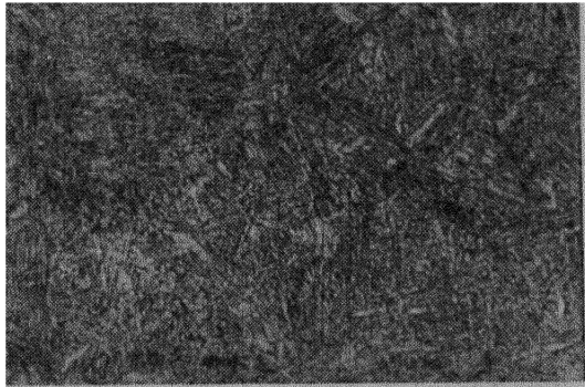
Fig. 202. Micrograph of superheated area in near-weld zone in steel 25X3HM after hardening and tempering (magnification \times 300 ).
