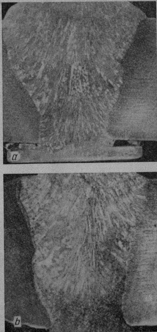
Fig. 258. Macrographs across welded joints made in reinforcing bars 60 mm in dia by the semi-automatic electric slag process:
