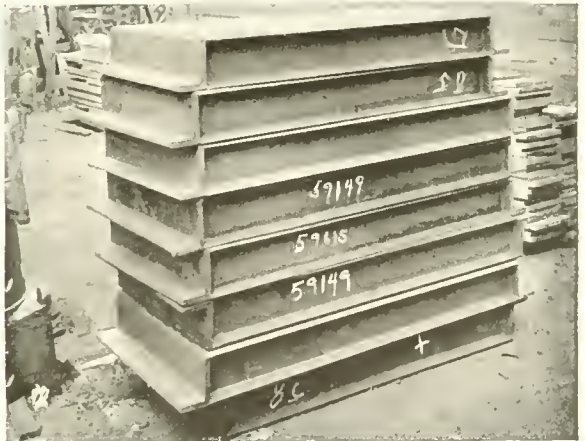
Fig. 99. Steel Machinery Bed-plates manufactured by use of Lincoln Arc Welder. Better and cheaper than a cast iron bed plate.
