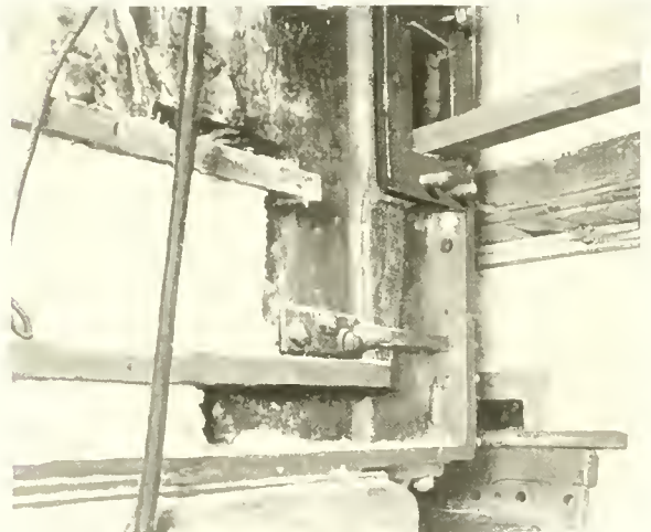
Fig. 64. Weld in intermediate cylinder of marine engine. (Courtesy BOOM BOILER & WELDING CO.)
