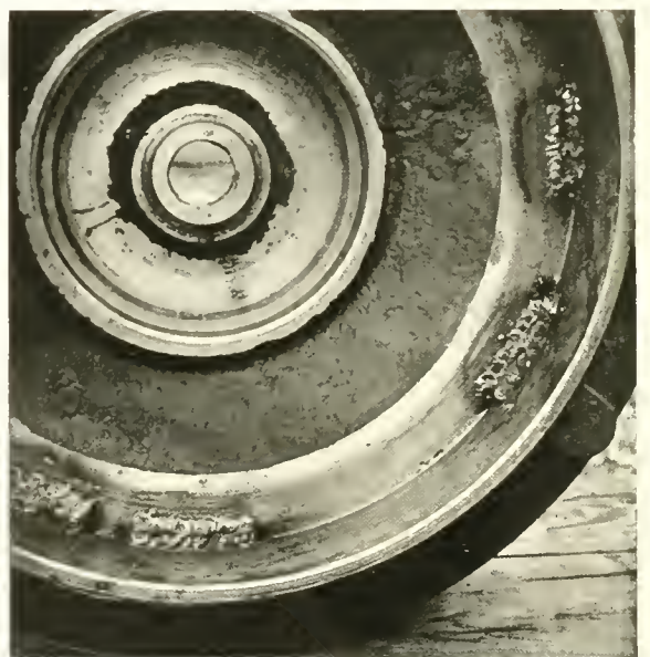
Fig. 17. Steel truck wheel casting (disk type). The defects in this wheel were found after machining had been done, and were perfectly welded and repaired with the Lincoln Arc Welder.
