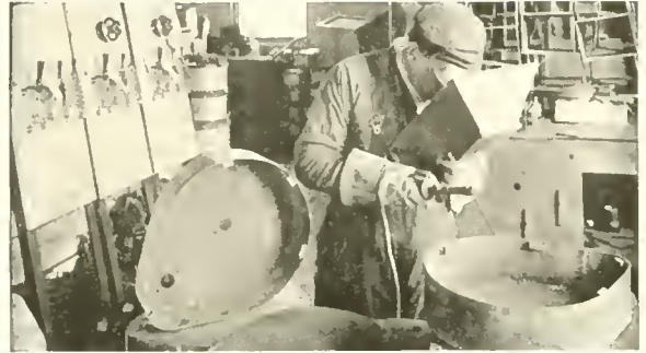
Fig. 89. Welding steel sheets together to form gear cases. The flanges on the inside of the case are also welded on. Jobs similar to this can be found in hundreds of manufacturing plants.
