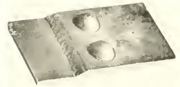
Fig. 104F. WELDING IN PLACE OF CALKING. Speed of work depends on amount of metal added. Strength of joint may be raised 25% doing the work at three times the welding speed given in table, page 6, for any thickness plate above 1/4". This makes a single riveted joint equivalent to a double riveted joint and makes a double riveted joint as strong as the original plate. Joints welded in this manner stand much abuse without leaking.
