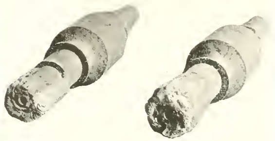
Fig. 102. Steel parts incorrectly machined built up by the arc welder and afterwards re-machined to proper size.
