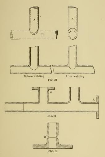
a hammer stroke on an iron flange brazed on an iron pipe results, in many cases, in a failure of the brazing. Oxyacetylene welding absolutely avoids this cause of possible accident, as there is no interposition of a chemically active metal.
