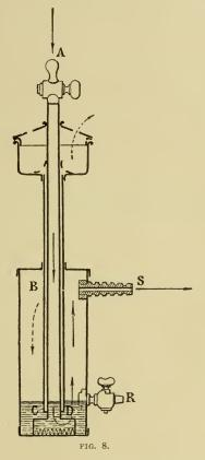
hydraulic safety valve. This appliance, Fig. 8, is composed of a central tube A for the combustible gas, terminated at its lower extremity by a bell-shaped casting, on the circumference
