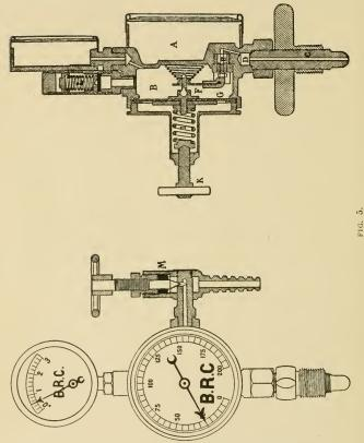
These gases, to be used in the blow-pipe, must therefore be brought to a lower pressure; this result is attained by the use of regulating valves mounted on the tanks. In the actual work these regulating valves are used in conjunction with gages, constantly indicating the pressure of the gas in the tank, and consequently how much gas is left in it.
