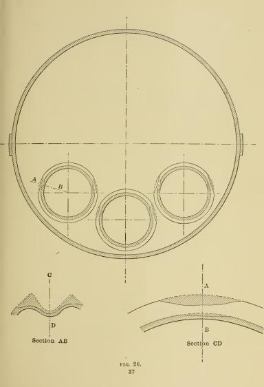
their original condition. In some spots they had been reduced by corrosion to a thickness varying between  $\frac{1}{16}$  and  $\frac{1}{16}$  inch.
