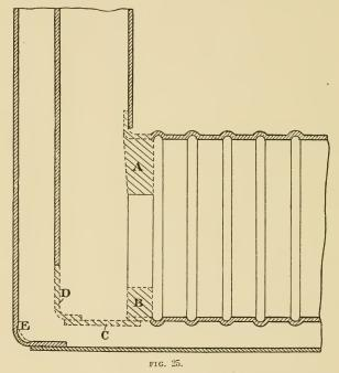
piece broke several times, but observations made in the case showed a defective quality in the plate to which the new piece was joined. The other fifteen held good. In the course of the work it was noted that the plates of the bottom of the boilers were badly eaten away at E on a space of about 36 inches; oxyacetylene welding was used to restore these plates to
