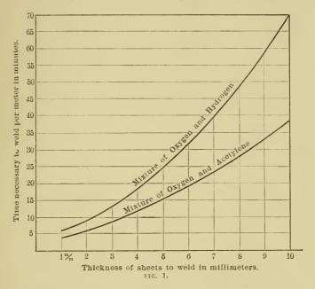
than in anything else, the regulating is of supreme importance, as the quality of the finished work is essentially dependent on it, because an excess of either the combustible or of the supporter of combustion may cause an alteration of the metal and its properties.
