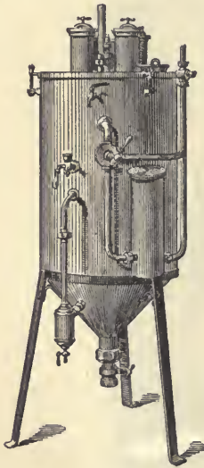
Fig. 34. — Generator for using the carbide in compressed cakes.
