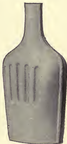
Fig. 222. — Aluminium water-bottle (military pattern) constructed by welding two stamped pieces.
