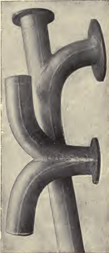
Fig. 217.—Red copper tubes entirely constructed by autogenous welding.
