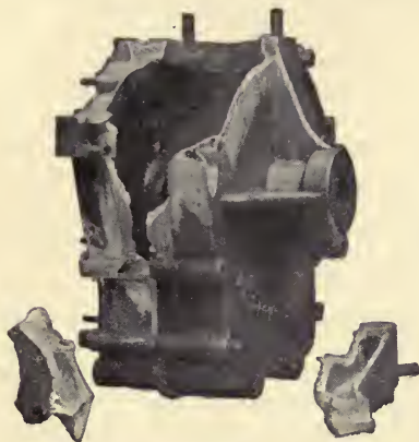
Fig. 226. — Gear-case, badly damaged.
