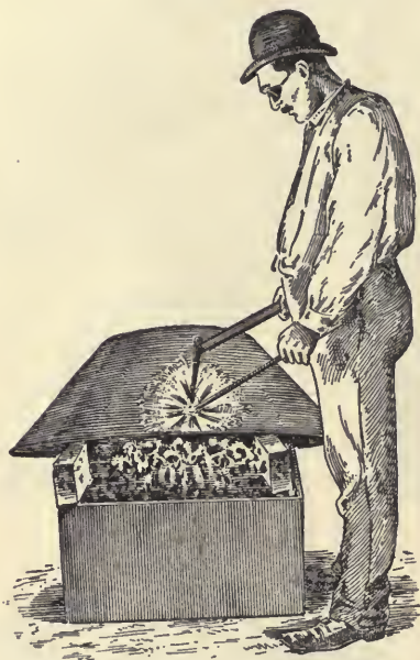
Fig. 210.—Repair of cast-iron vat whilst on the fire.
