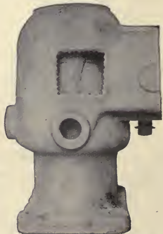
Fig. 205. — Repair on a motor cylinder executed on the interior surface. A piece has been cut from the water jacket opposite the crack, and will afterwards be replaced by welding.
