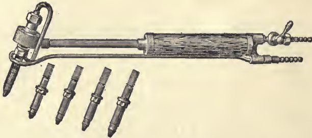
Fig. 52.—Cyclop blowpipe with interchangeable heads.
