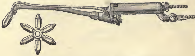
Fig. 57.—Picard blowpipe with the oxygen regulator.
