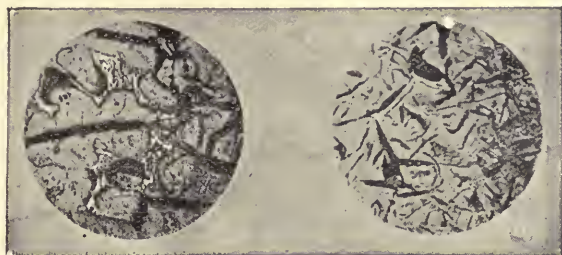
Fig. 195.—Microphotographs of two samples of grey cast iron; notice the particles of carbon in the free state.
