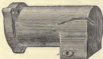
Fig. 197.—Cast-iron object bevelled previous to welding.
