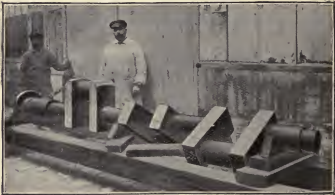
Fig. 190.—Repair of crank-shaft.
