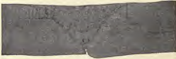
Fig. 175.—Weld of mild steel executed without bevelling; adhesion and interposition of oxide (photograph after corrosion test).
