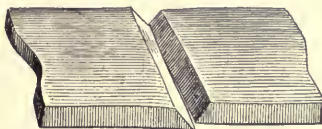
Fig. 92.—Overlapping of the bevel, which should be avoided.
