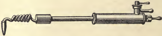
Fig 13.—Oxy-coal gas blowpipe ("Claude" system).
