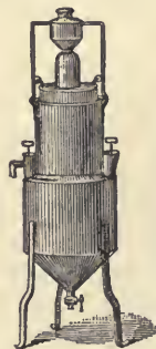
Fig. 28.—One type of granulated "carbide to water" generator.
