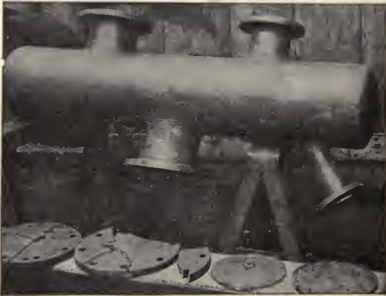
Fig. 189.—Vapour collector made by autogenous welding. Tested hydraulically the plates closing the branches were fractured but the welds unaffected.
