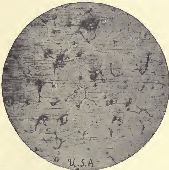
Fig. 223.—Microphotograph of an aluminium-zinc weld (gear-case metal) executed without cleaning flux; numerous layers of alumina in the metallic mass.
