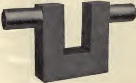
Fig. 252.—Crank-shaft cut by the cutting blowpipe from a plate.
