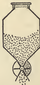
Fig. 29.—Distribution of granulated carbide by bucket wheel.
