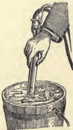
Fig. 62.—If the blowpipe is cooled by immersion in water, the oxygen should not be completely shut off.
