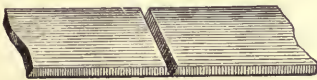
Fig. 90.—Bevelling for pieces from \frac{1}{8} inch to \frac{3}{16} inch in thickness, angle of bevel 45^\circ .
