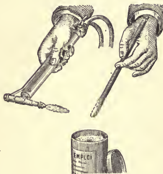
Fig. 198.—The extremity of the welding rod, previously heated, is dipped into the cleaning flux.
