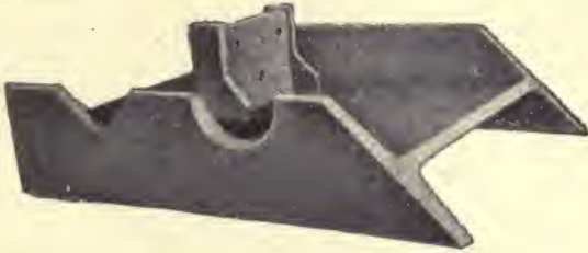
Fig. 253.—Piece completely executed by cutting blowpipe.
