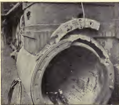
Fig. 208.—Locomotive cylinder badly damaged. Replacing it would have cost £160.
