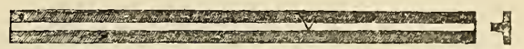
Figure 6 is the tongued iron secured to the inside upper edge of the carriage body, and on which figure 5 slides.
