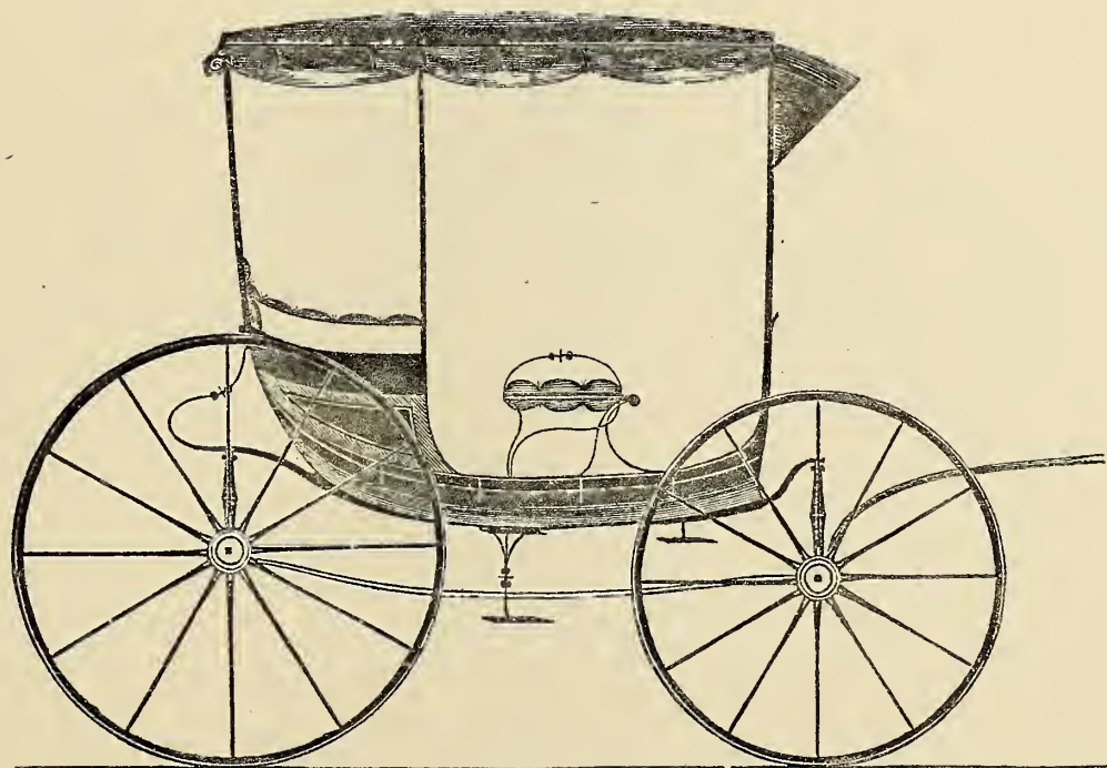
ROCKAWAY WITH TURNOVER SEAT.— \frac{1}{2} IN. SCALE.
