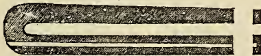
Figure 5 is a view of the irons attached to the inside lower edge of the seat, in which iron is the groove that sustains the seat and keeps it from defacing the plating on the edges of the carriage body.
