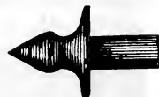
Form of Pin before welding, to be made in half collar tool.
