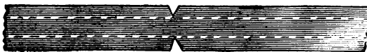
Fig. 164—Plain Bar with Four Bars Welded Upon It, Leaving Gaps at Center.
