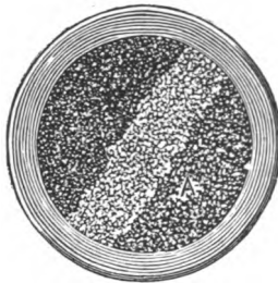
Fig. 162—Front Axle of Fire Engine. Dark Portions Show Old Cracks, Light Band the Final Break.
