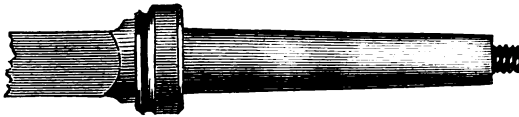
Fig. 166—Axle with a Sharp Corner at the Point where Arm and Collar Meet.
