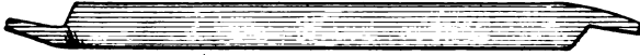
How to Make a Pair of Common Tongs. Fig. 9—Shape to which "J. M. W." would Draw the Iron.
