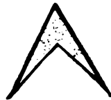
Fig. 385—Showing the Steel After it has been Cut into and Doubled Around.
