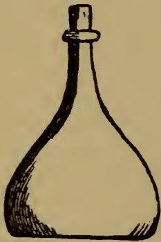
FLORENCE FLASK, used in gener- ating chlorine gas.
