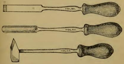
TOOTH CHISEL, RASP AND HAMMER.
