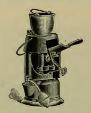
The Furnace, as arranged, is absolutely non-explosive, being provided with an air-blast, which supplies the necessary pressure to force the fluid to the burner, instead of the elevated tank.
