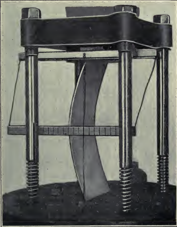
FIG. 11.—A PLYWOOD COLUMN READY FOR TEST.
