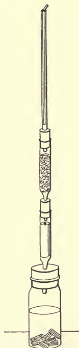
FIG. 98.—The apparatus for the determination of arsenic.
