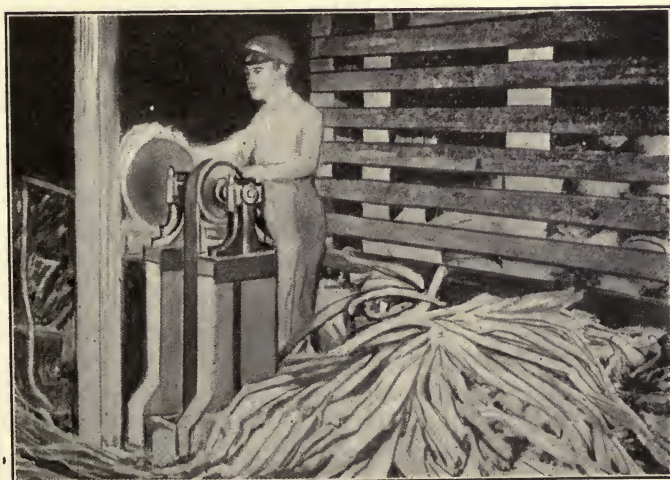
FIG. 63.—Wooden spool for rolling into coils. (By permission of the Bureau of Fisheries, Washington, D. C.)
