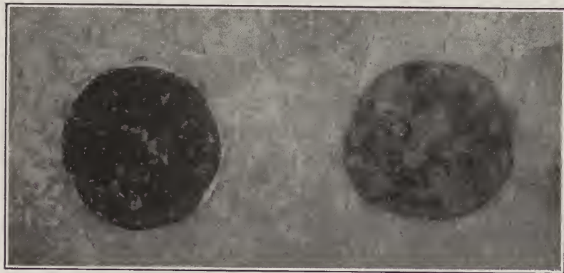
FIG. 41 SPOT TEST ON GALVANIZED IRON Showing Etching Effect of Basic Pigments
