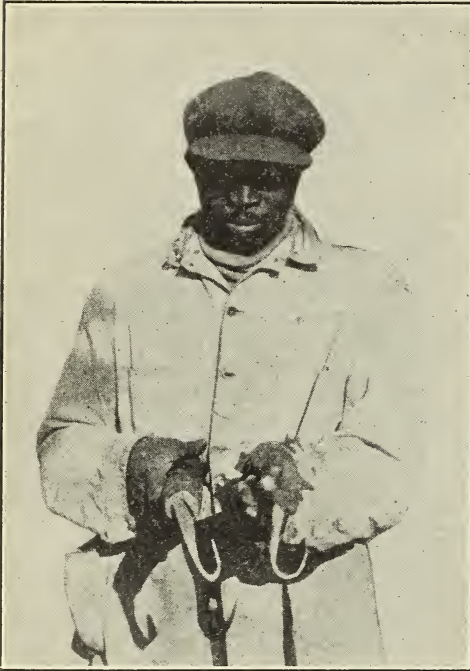
FIGURE 1.—For \frac{3}{4} -inch chipping small hacks (left) are preferable to the "broad-billed" hacks (right) formerly used
