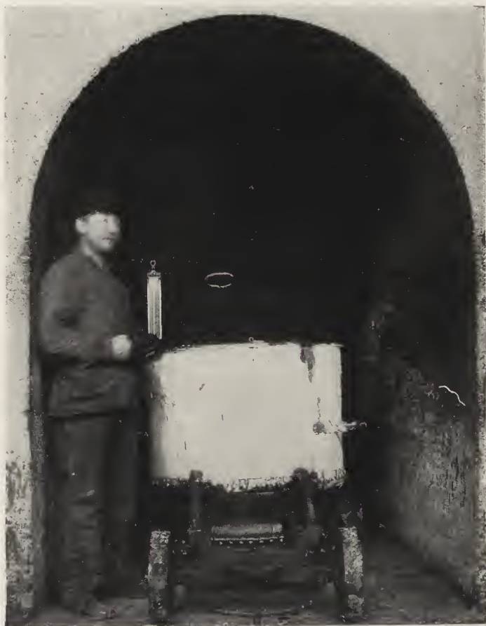
FIG. 35.—Cooking the Oil and Resin Together.
