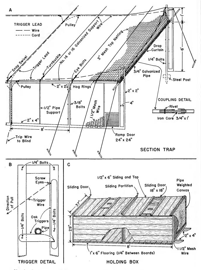
Fig. 3.--Construction details for drop-cuftain type section trap and for holding box.
