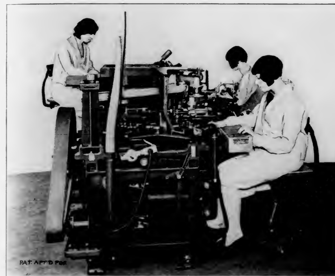
View of the New Universal Model R Rolling Machine in Operation in conjunction with the Model S Long Filler (non-blending type) Bunch Machine, which is shown in the rear.
