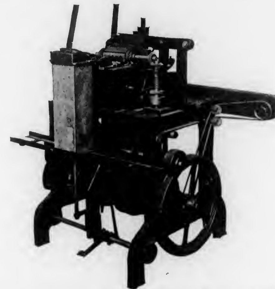
Automatic Bunching Machine, Bunches 22 Cigars a Minute
