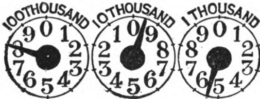
FIG. 11.—Gas meter—index reads 79,500 cubic feet.
