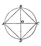
40. By bisecting the arcs AB, BC, CD, and DA, and joining the points of bisection, we can form an octagon; and by bisecting the arcs which subtend the sides of the octagon, we can inscribe a polygon of sixteen sides.
