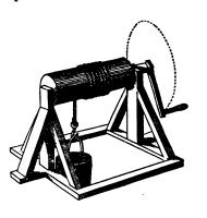
The power to the weight, as the radius of the axle, to the length of the crank, or radius of the wheel.
