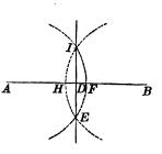
Then join the points I and E by the line IE: the point D where it intersects AB, will be the middle of the line AB.
