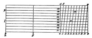
10. This scale is thus constructed. Take ab for the unit of the scale, which may be one inch,  $\frac{1}{2}$ ,  $\frac{1}{4}$  or  $\frac{3}{4}$  of an
