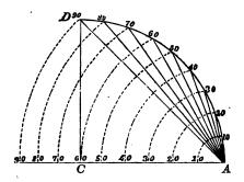
11. If, with any radius, as AC, we describe the quadrant AD, and then divide it into 90 equal parts, each part is called a degree.
