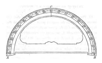
13. This instrument is used to lay down, or protract angles. It may also be used to measure angles included between lines already drawn upon paper.
