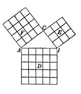
AB be equal to the sum of the squares E, and F described on the sides CB and AC. This is called the carpenter's theorem.
