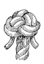
Fig. 126.—Double wall and crown.
