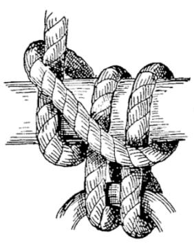
Fig. 51 A.—Roband hitch (front).
