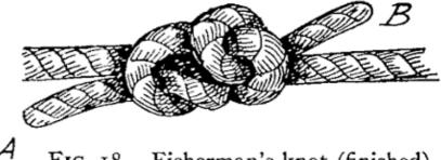
Fig. 18.—Fisherman's knot (finished).
