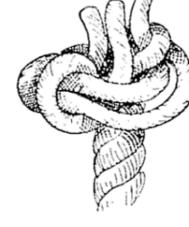
Fig. 121 A.—Making double crown.
