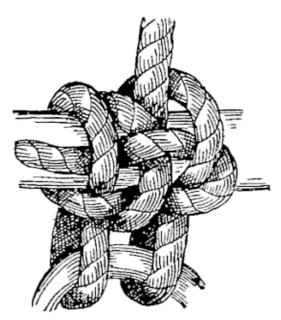
Fig. 51 B.—Roband hitch (back).
