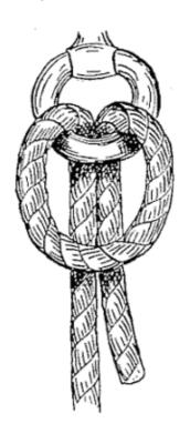
Fig. 31.—Lark's head with toggle (A) withdrawn.
