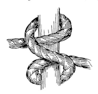
Fig. 36 A.—Clove hitch or builder's hitch (tying).
