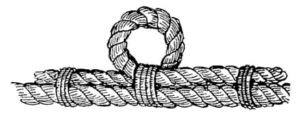
Fig. 96.—Lashed cut-splice.
