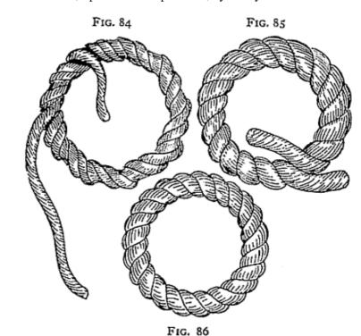
Figs. 84, 85, and 86.—Grommet complete and making.
