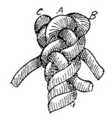
FIG. 112.—Single crown tucked (making).
