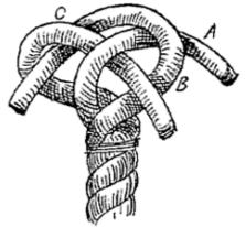
Fig. 111.—Single crown (making).
