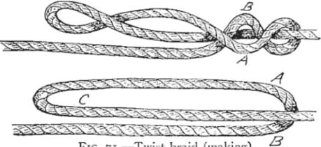
Fig. 71.—Twist braid (making).
