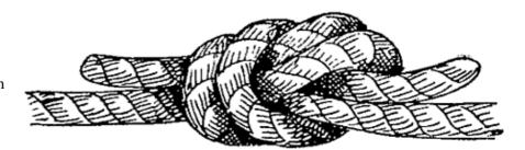
Fig. 19.—Ordinary knot (finished).
