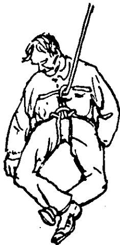
B. The Spanish bowline used to lower an unconscious person
