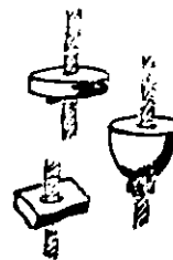
Figure 202 Types of Chocks
