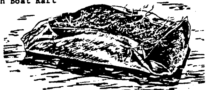
Figure 295 The Brush Boat Raft
