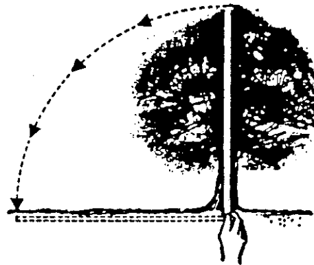
Figure 352 Lumberman's Method of Determining Heights
